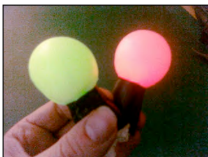
Figure 10. Ping-Pong LED balls for colour tracking.
