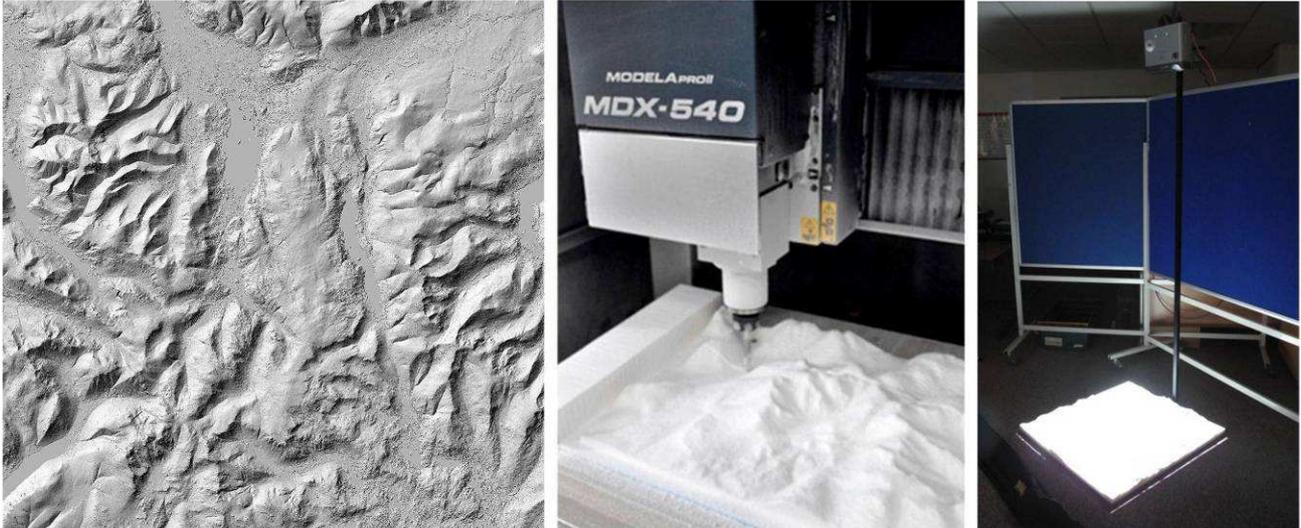
**Figure 4.** Creating the PARM prototype: Hillshade view of the DSM of Cumbria (left); The milling of one tile (centre); The prototype PARM system (right).
