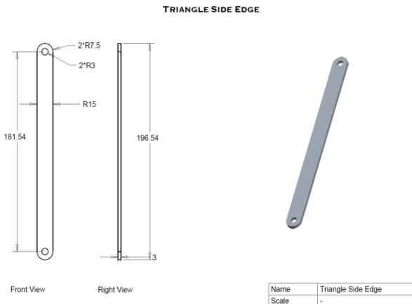
**Figure 2: Triangle Side Edge – Basic Dimensions**
