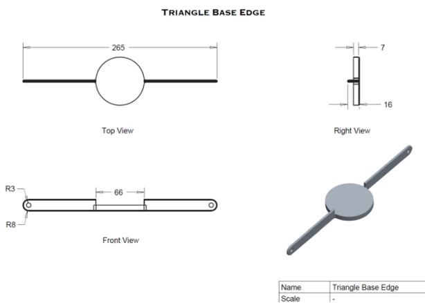
**Figure 3: Triangle Base Edge – Basic Dimensions**
