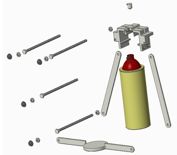
**Figure 5: DDArtS V2 – Exploded view of the assembly**
