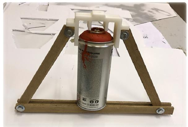
**Figure 6: DDArtS V2 prototype – Printed Main Frame and wooden Side and Base Edges**
