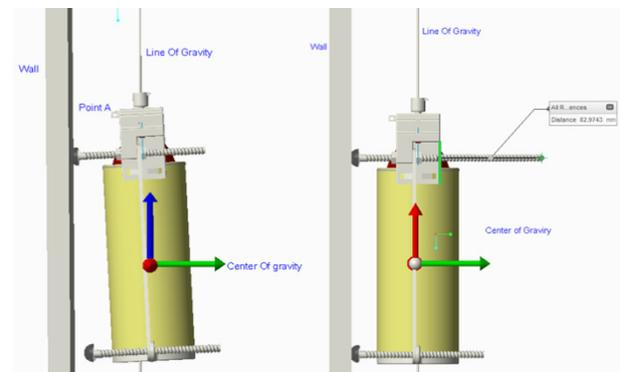
Figure 9: Unstable Equilibrium due to resultant force on Point A (left) – Stability Equilibrium while on motion (after the optimisation test) (right).
