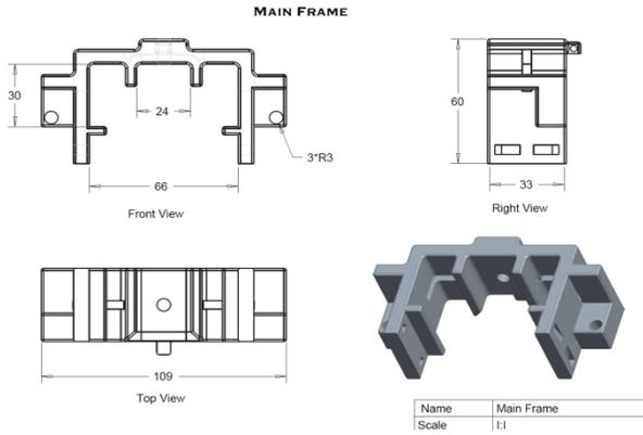
**Figure 1: Main Frame – Basic Dimensions**
