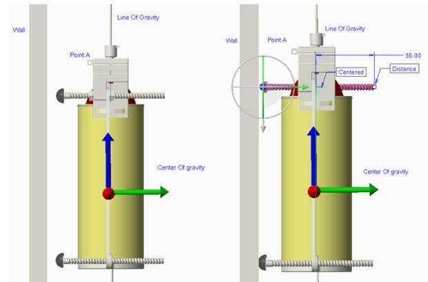
Figure 8: Stability Equilibrium at rest (no motion)
