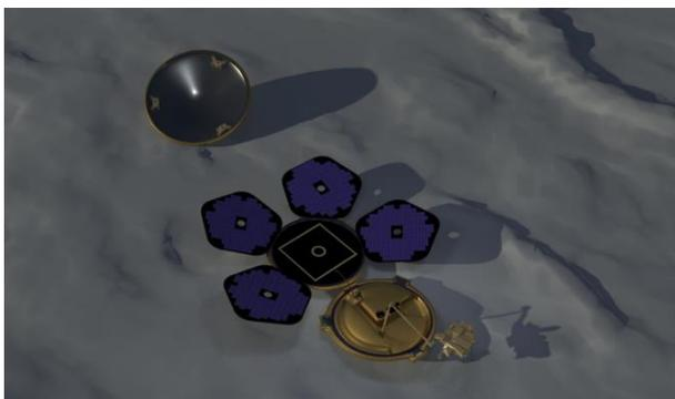
**Figure 3:** Lander with four panels and robotic arm deployed, heat shield and terrain (WIP render)
