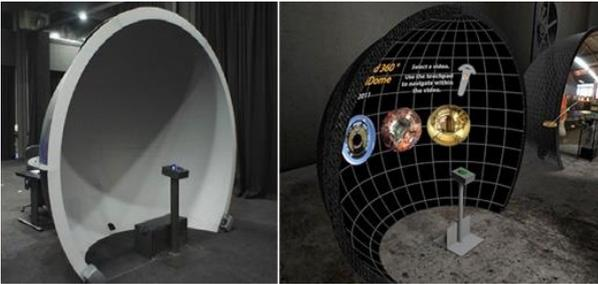
**Figure 6:** iDome trackball user interface for gaze control within spherical imagery. Photograph (l), 3D model (r).
