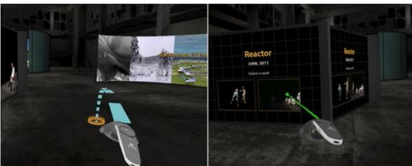
**Figure 7:** Locomotion outside the tracking area in VR with controller and teleportation (l). Selection of a work in VR with controller and virtual laser pointer (r).
