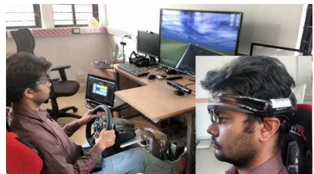
Figure 1: Participant wearing Tobii glasses and EEG tracker and the Kinect placed on the table
